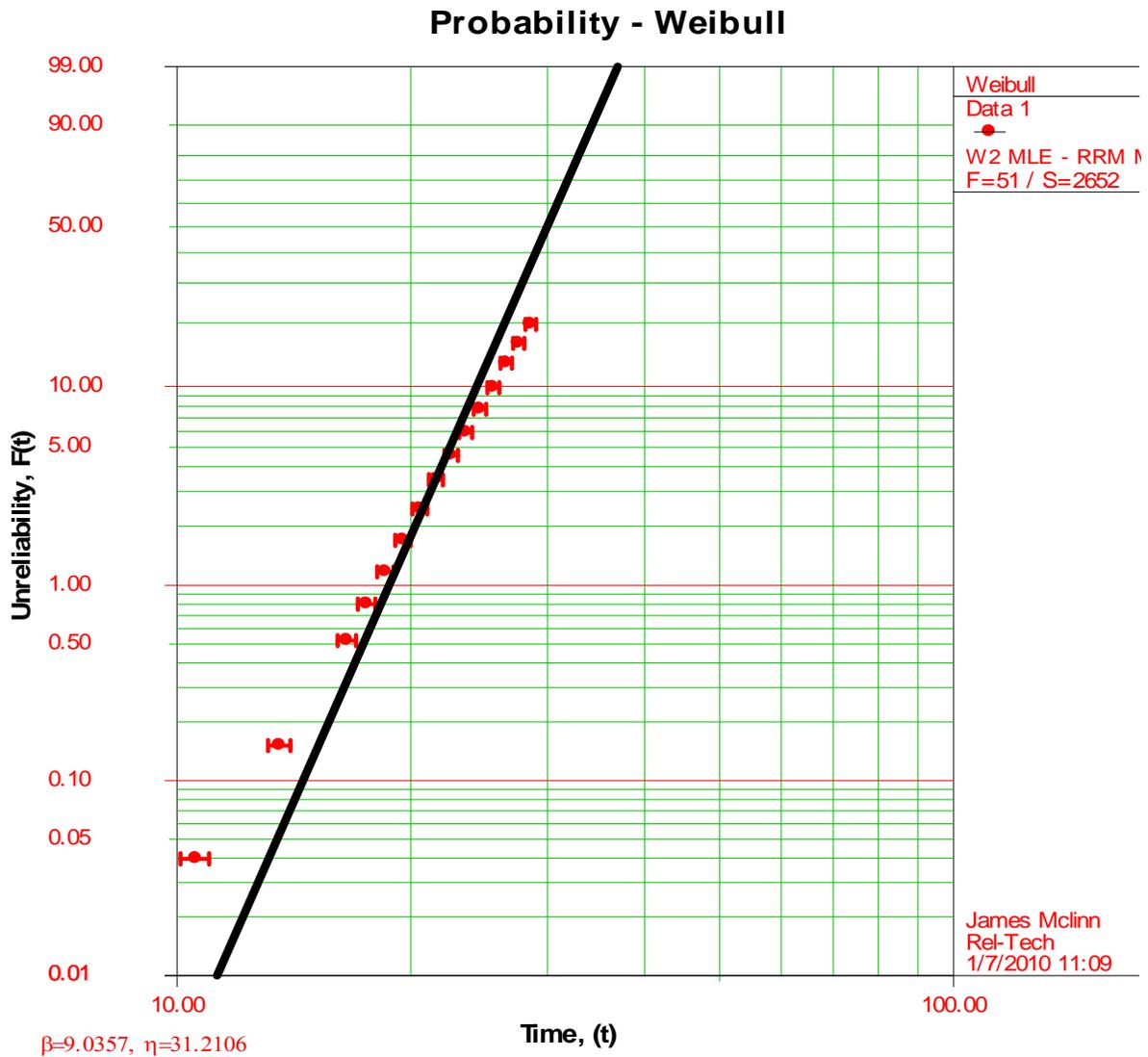
**Fig. 16 – Voltage Regulator Field Data**
