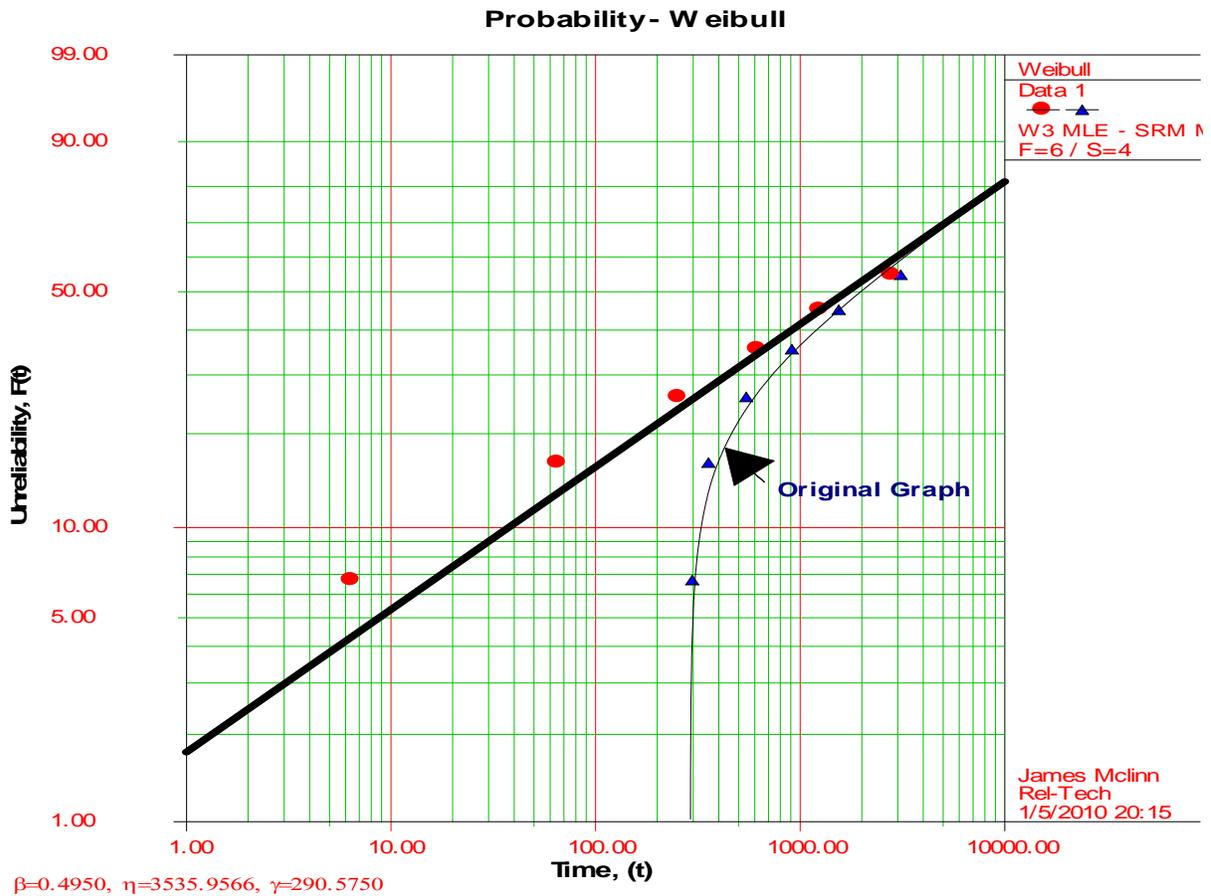
**Figure 5 - Three Parameter Data Transformed**
