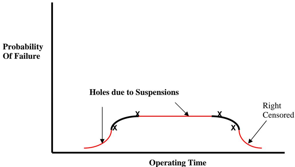
**Figure 12- The Suspensions as Holes in the Probability Distribution**
