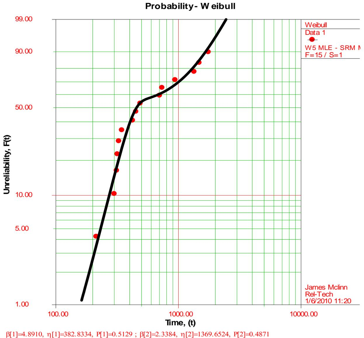
**Figure 14 – Mixed Failure Modes from an ALT of RAMs**
