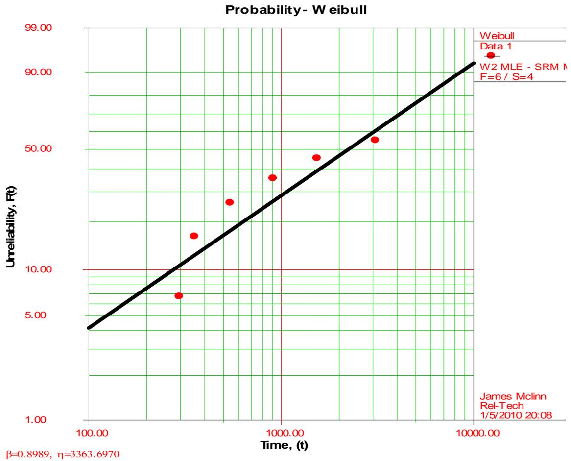
**Figure 4 - The Curved Data on a Weibull**
