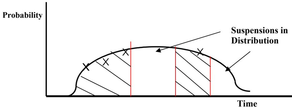
**Figure 18 - Time to Failure with Suspensions**
